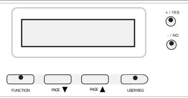
The Function mode is used to set up or to adjust various parameters related to the operation of this keyboard. With the FUNCTION button engaged you may access the menu for the Touch, Metronome Volume, Split Point, Reverb level, Layer Reverb Level, Lower Reverb Level, Chorus level, Layer Chorus Level, Lower Chorus Level, Song Volume, Octave, Layer Octave, Lower Octave, Pedal Assign, Master Tune and Grade selections.
